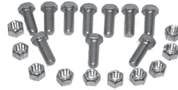
Support Leg Bolt Kit 700-50-35 Contains: 10-5/8" x 1-3/4" Grade 8 Bolts 10-5/8" Lock Nuts
