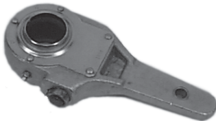
17-A23-66B 37-Spline; 1-5/8" 6" Drilling
