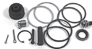
Slack Adjuster Kit (Minor) RW-KIT963
